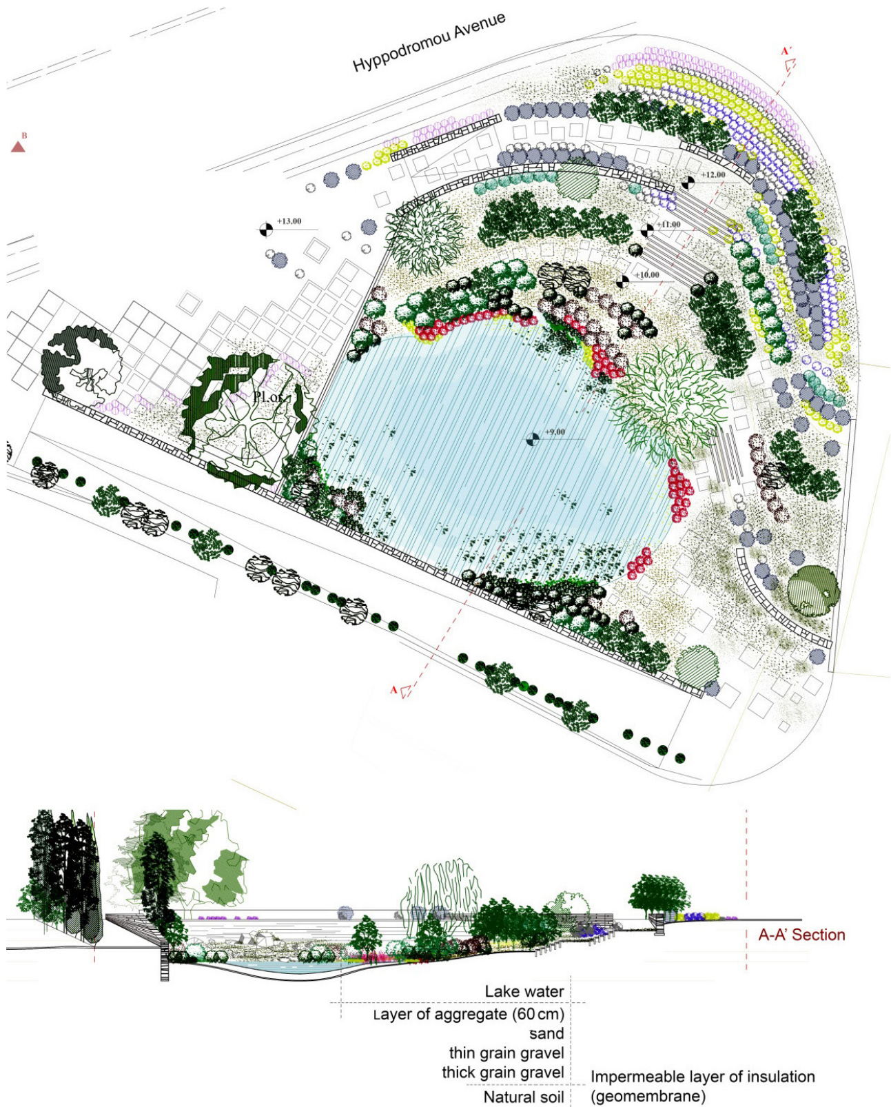
Figure 12 Ground plan and section A-A' of the wetland at the entrance of the area Source: Design by the authors
